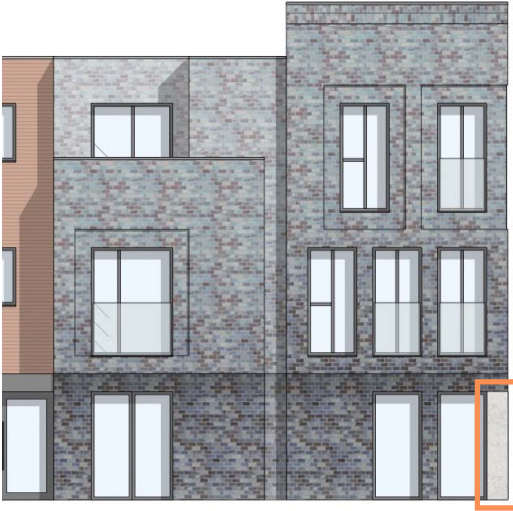
Pre-cast corner element on both blocks
